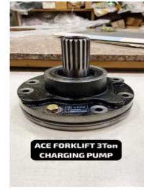
ACE FORKLIFT 3TON CHARGING PUMP
